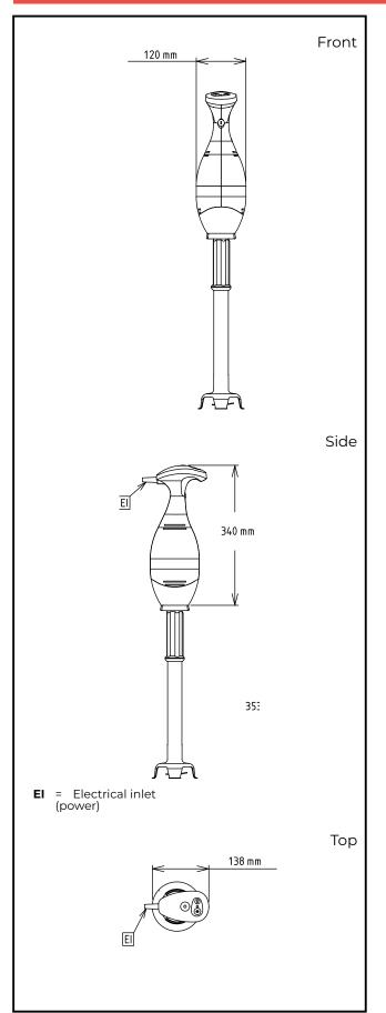
Electric Supply voltage: 220-240 V/1 ph/50/60 Hz **Electrical power max.:** 0.75 kW 0.75 kW **Total Watts:** Capacity: Capacity (up to): 270 Litre Key Information: External dimensions, Width: 138 mm External dimensions, 120 mm Depth: External dimensions, Height: 865 mm **Shipping weight:** 4.8 kg
